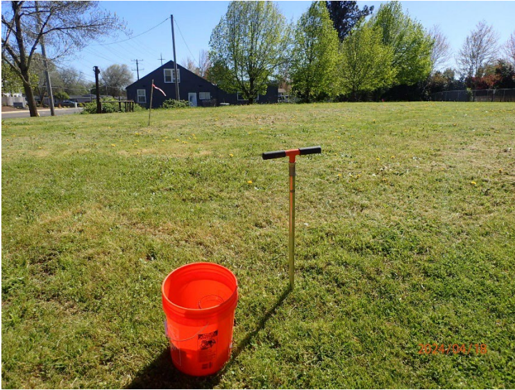
View east showing stainless-steel sample probe used for surface soil collection at decision unit DU01.
