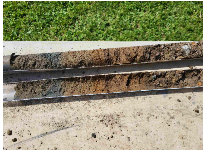
Bored material was mostly fine-grained down to approximately 17 feet, where coarser material was encountered.
