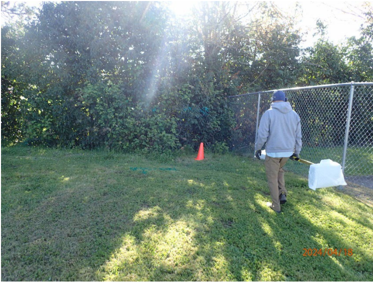
An electro-magnetic scanner was utilized to screen for the presence of buried objects.
