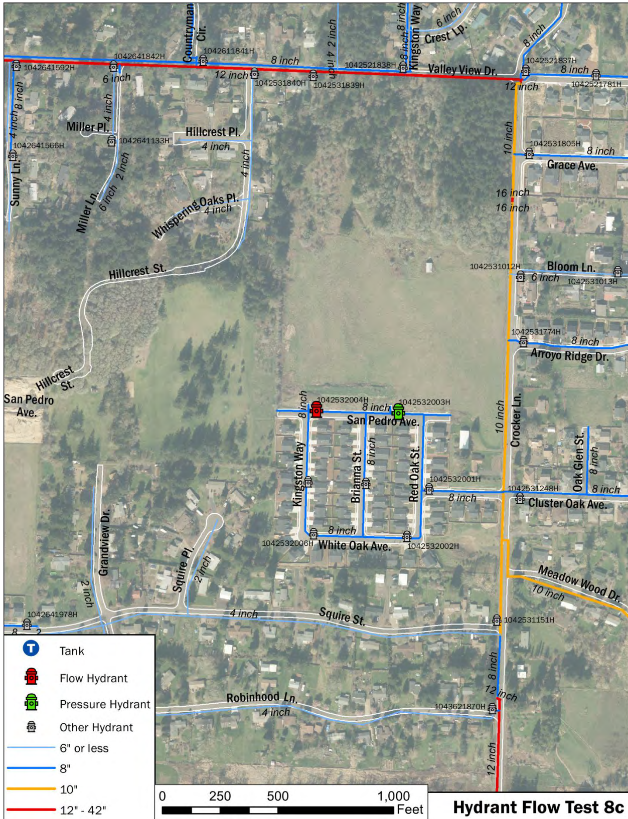
Figure A-10. Hydrant Flow Test 8c Map
