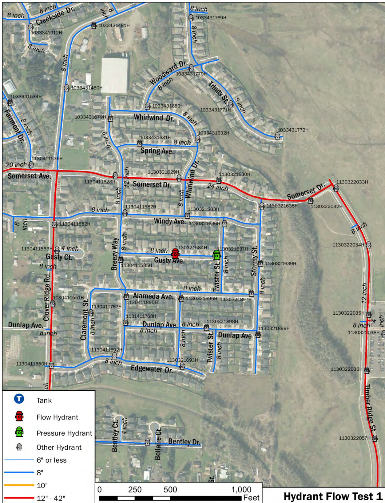
Figure A-1. Hydrant Flow Test 1 Map
