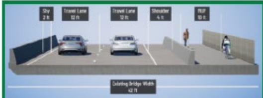
Section 2-2 Alternative 2F - Bridge deck reconfiguration
